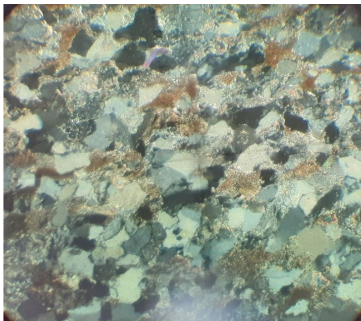
Figure 2 – Outburst-hazardous sandstone d_3Sd_4 from the Pokrovsk mine, coastal marine facies, fine-grained, sorted, weakly rounded, little altered, thin section, magnification 100^{\times}
